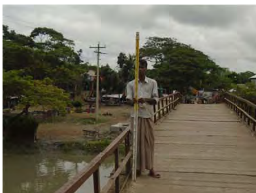
Picture 2.7:Water level gauge connection with Ckhinikandi Bridge TBM using Level machine
