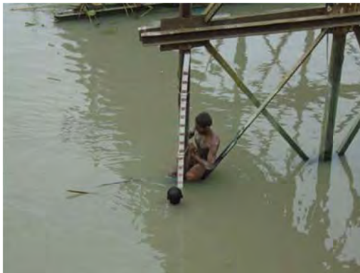
Picture 2.5:Water level gauge at D/S of Chiknikandi Bridge
