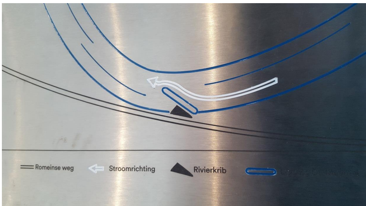
Figure A.1 Archeological reconstruction of a Roman groyne at De Meern near Utrecht, the Netherlands. The groyne was made of basalt stone and wood. Its purpose was to protect a road against bank erosion.
