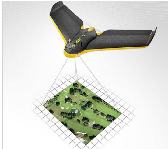
Figure 4: Picture of the Ebee of Sensefly, a small plane (1 meter wide, 0,7 kg), which can produce digital elevation models for up to 10 km 2 in a single flight with an accuracy of 5 cm.
