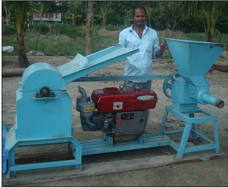
Pic. 11a. Semi-automatic fish feed pellet machine (Diesel operated 16 HP semi moist pellet @250-300 kg/hr)
