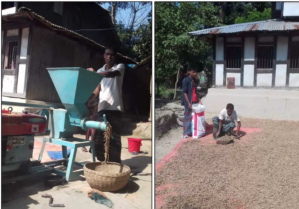
Pic. 11b. Fish feed pellet machine was being operated one of the project beneficiary.
