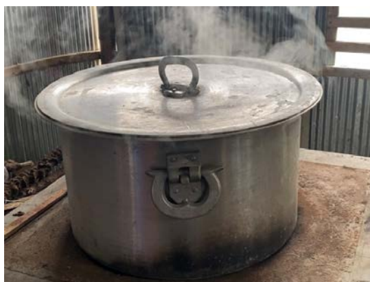
Fig. 15-2. Cooking of water hyacinth stalks with water and potassium hydroxide
