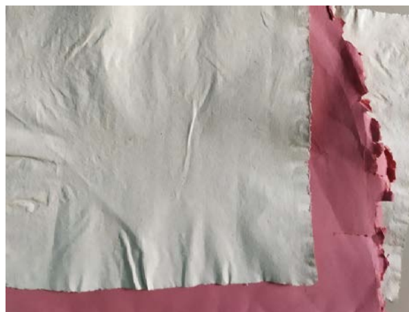
Fig. 15-6. Final hand sheet from water hyacinth
