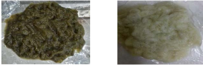
Fig. 11. Unbleached (left) and bleached pulp (right) made from water hyacinth
