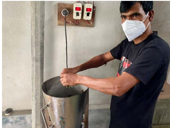
Fig. 15-3. Disintegration of pulp using a blender
