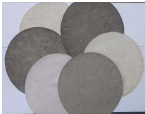
Fig. 12. Handmade paper made from bleached (light) and unbleached pulp (dark)
