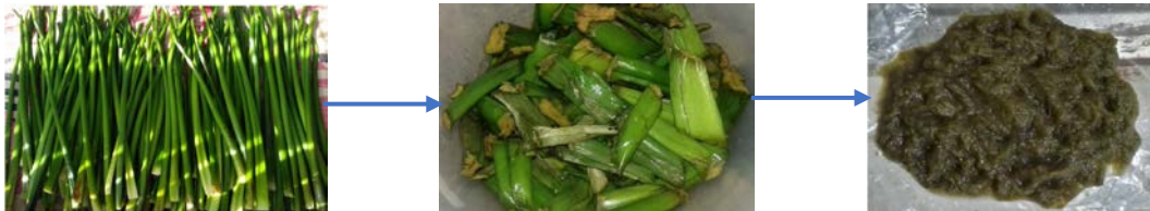
Fig 10. Pulp produced from fresh water hyacinth stalks
