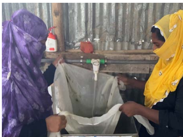
Fig. 15-4. Washing of pulp after bleaching
